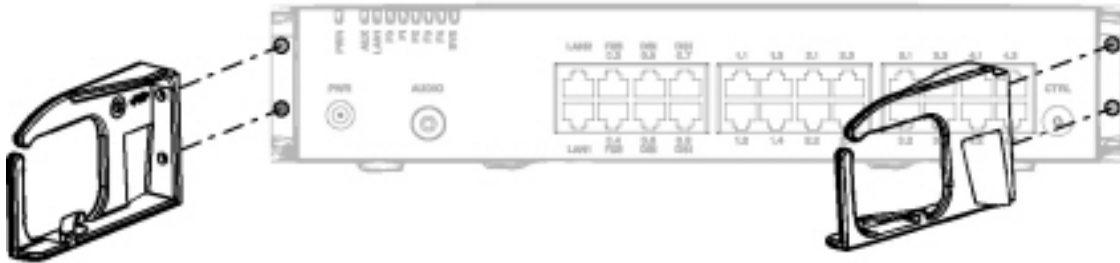
Figure 17: Installing the brackets for the cable cover
